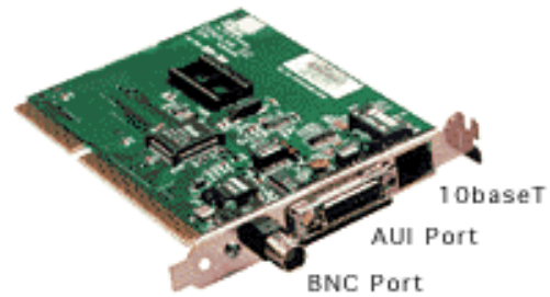
Typical ethernet card showing the three common types of connectors
